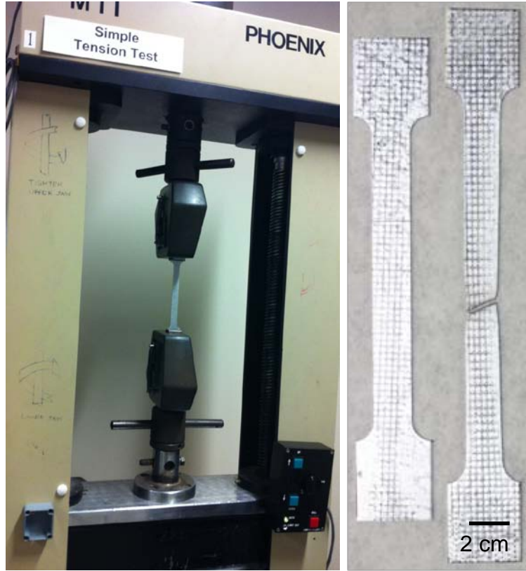
Figure 17: Specimens before and after tensile test.
