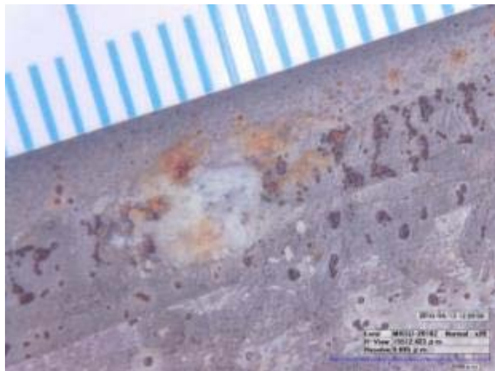
Figure 32: Pits and corrosion product at ribbed regions of an in-situ SRAP specimen in S + solution after ~300 days of exposure. 1 mm markers (specimen internal ID code: Bin 7 R8).
